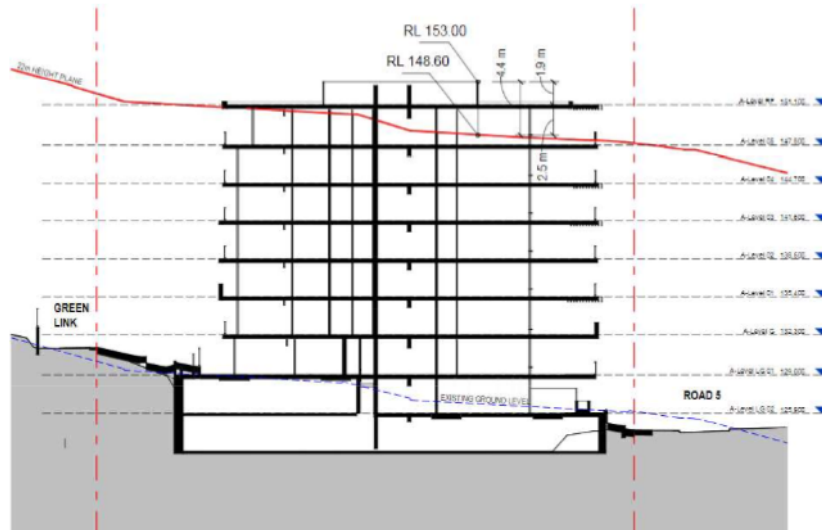
Figure 4 South Section of Building A showing the extent of height contravention (4.4m) (Source: Mirvac Design)
